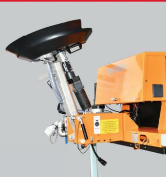
**Fold-up spreading device**
