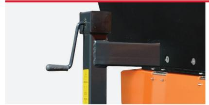
**Mechanical parking system with hand crank for unloaded spreaders**
