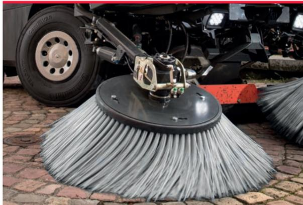
The brush arms include forward impact shock absorbers and side impact hydraulic dampening to reduce damage costs. A replaceable "Shear Pin" which can be easily replaced by the operator, protects the brush arms and chassis from expensive repairs.
