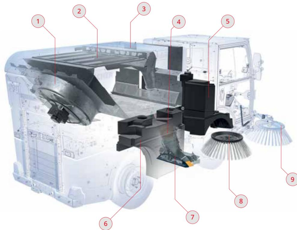
**1** Optimised fan arrangement, with bigger, optimised blade wheels for greater efficiency
