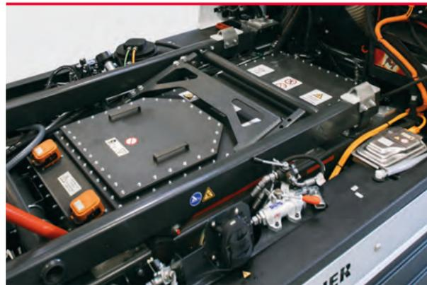
Specially designed Bucher Battery Pack with superior lifetime and minimal memory effect. Made with high quality automotive prismatic Li-ion NMC cells, managed through an automotive battery management system, the battery is placed in a shock, water and dust-proof case. The Bucher Battery Pack is maintenance-free and has a sophisticated repair concept for maximum safety. Due to the electric drive concept of the sweeper, maintenance and service costs in general are kept low.
