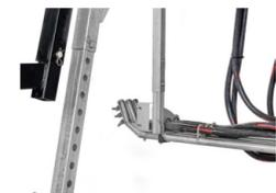
**Spray nozzle bars with height adjustment**
