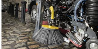
This option provides infinite control of the channel brush lateral position from the cab mounted door controller, allowing the operator to easily achieve the best cleaning position.
