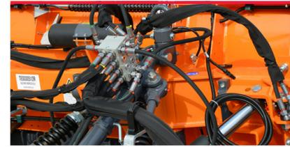
**Patented self-adjusting bypass valve**
