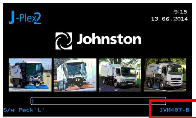
**Figure Three: Controller Type**
